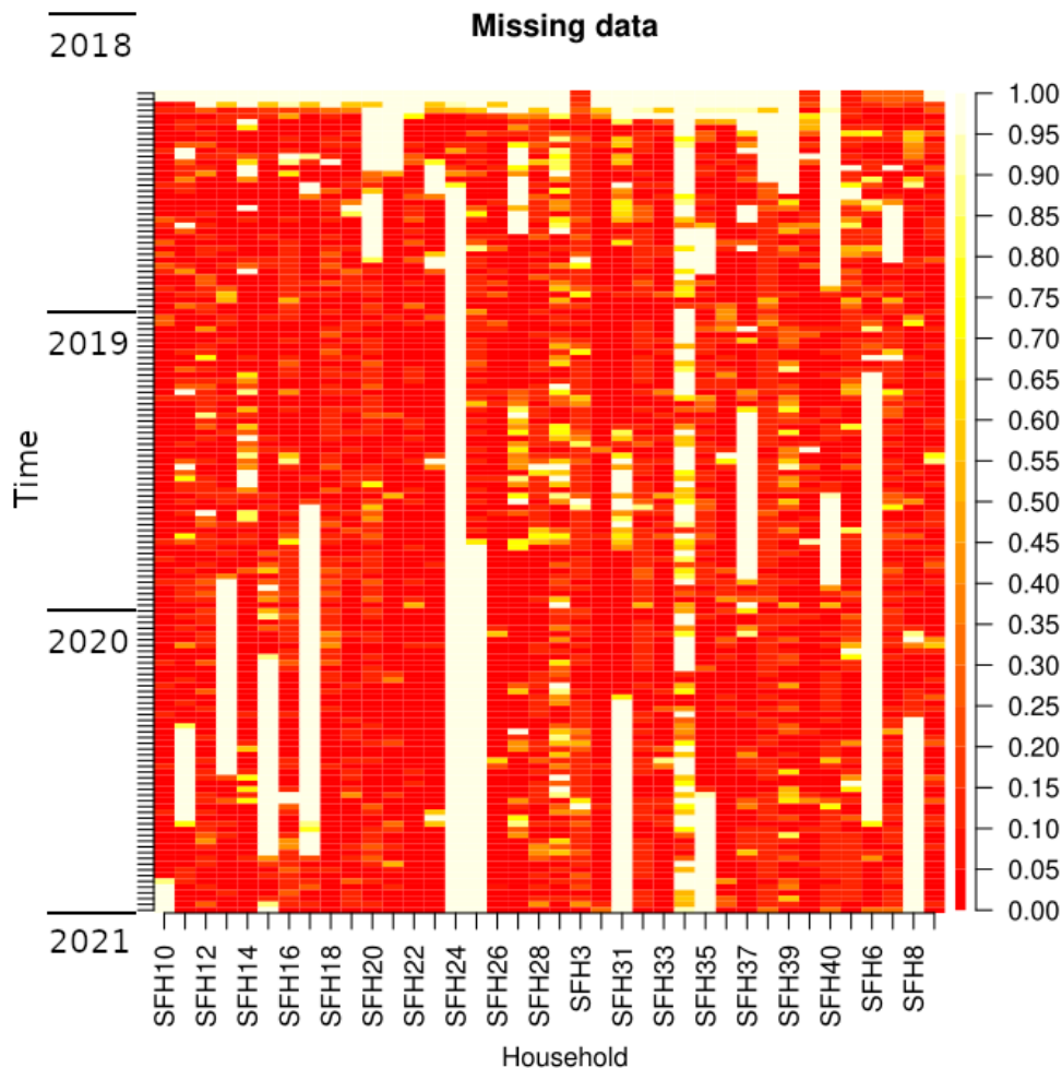
Figure 2: Fraction of missing data in pump power consumption for each household over time (aggregated per week). Light areas indicate large fractions of missing data. Note that the households are sorted alphabetically: SFH10-SFH30, SFH3, SFH31-SFH40, SFH4-SFH9.
