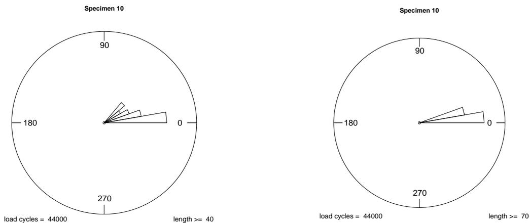
Figure 14: Orientations of the cracks after 44000 load cycles. Left:  $\text{length} \geq 40$ ; Right:  $\text{length} \geq 70$
